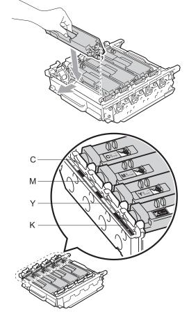
C - Cyan M - Magenta Y - Yellow K - Black Make sure the green lock lever (1) is in the release position as shown in the illustration.
